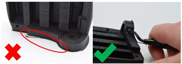
**Fingertip Casting:** Check to see if any of the fingertips contain unacceptable defects. If any of the following are present, throw out the part and use a different one:
