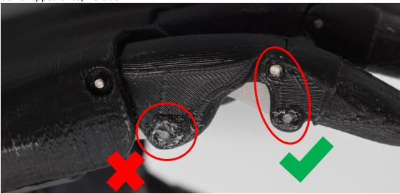
**Smooth Opening and Closing:** Open and close the hand and observe to ensure that the hand opens and closes fully. This can also be tested by pulling on the cable on the harness. Look for any friction while the hand is moving. The hand should spring open very easily.
