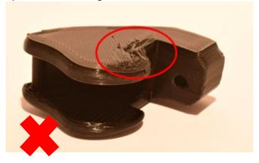
**Brim and Supports:** Check to ensure that the brim and supports are removed. If they are not, remove them with pliers or a deburring tool and file to smooth.
