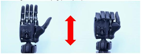
**Backlock:** Test the hand with the backlock button in both the "locked" and "unlocked" positions. Ensure the following:
