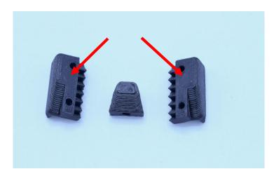
**Thumb Rotation:** Ensure that the thumb moves when pushed. If it is too difficult to move, loosen the screw. If it is falling without any force, tighten the screw.
