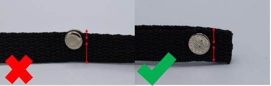
• Ensure that both halves of the rivet are fully flattened together. If it is not, use large pliers and apply more force.
